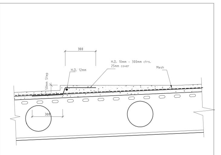
50mm STEP IN SLAB (STEP PERPENDICULAR TO JOISTS)
